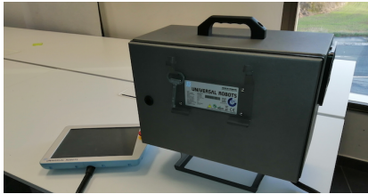
(a) Universal Robots UR3 robot CB3.1 controller and associated teach pendant (HMI). The controller has a generic mechanical lock aimed to secure physically access.
