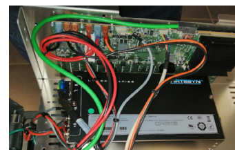
C) The main computer of the controller and the PSU are affixed to the front plate. Given the real state available we miss some cable management.
