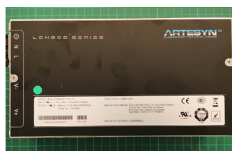
E) The PSU is a Artesyn LCM600 series with an output of 48 V, and an input of 85–264 Vac. Has a typical full load efficiency of 89% up to 600 watts.
