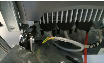
G) The on-board controller is the embedded and “ruggedized” EC70A-SU from DFI which features an Intel processor and a Ubuntu 16.04 file system.
