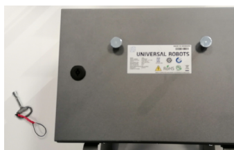
A) Universal Robots UR3e controller. The controller has a mechanical lock aimed to prevent ingress to the internals from non authorized parties.
