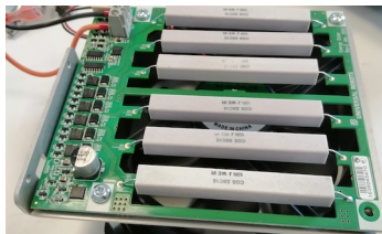
G) The energy-eater board. This component tends to overheat a fair bit and should generally be checked in case of failure for signs of degradation.
