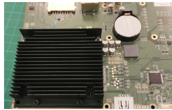
H) Under the heatsink we find a MSC Q7-BT module on an ECX form factor and an Intel SoC with DDR3L memory.
