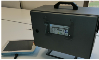
A) Universal Robots UR3 robot CB3.1 controller and associated teach pendant (HMI). The controller has a mechanical lock aimed to secure physical access.
