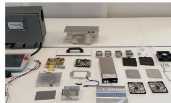
I) Final figure depicting all the components contained inside of the Universal Robots UR3CB3.1 controller, leaving aside the teach pendant.
