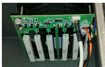
D) The energy-eater board. This component tends to overheat a fair bit and should generally be checked in case of failure for signs of degradation.
