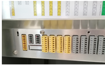
E) The safety side of the controller (documented in the user manuals) includes quick connectors which can be removed by carefully wiggling them out.
