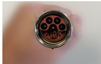
K) Even though the pin-out is quite similar to previous iterations of the CB3 controller, the connector itself has a different shape.
